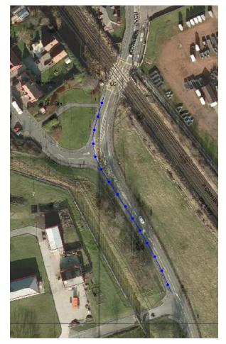
Figure 1: This diagram shows the route of the approach to the signal. A driver moves from bottom to top. The signal is at the top of the diagram. The dots mark points that are spaced at 10m apart along the route.
