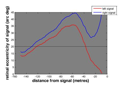
Figure 6: This graph shows how far out into the periphery of vision the image of the left hand (nearside) and right hand (offside) signals falls on approach to the signal. It is assumed that a driver is 2m from the kerb and looking at a point 10m ahead.
